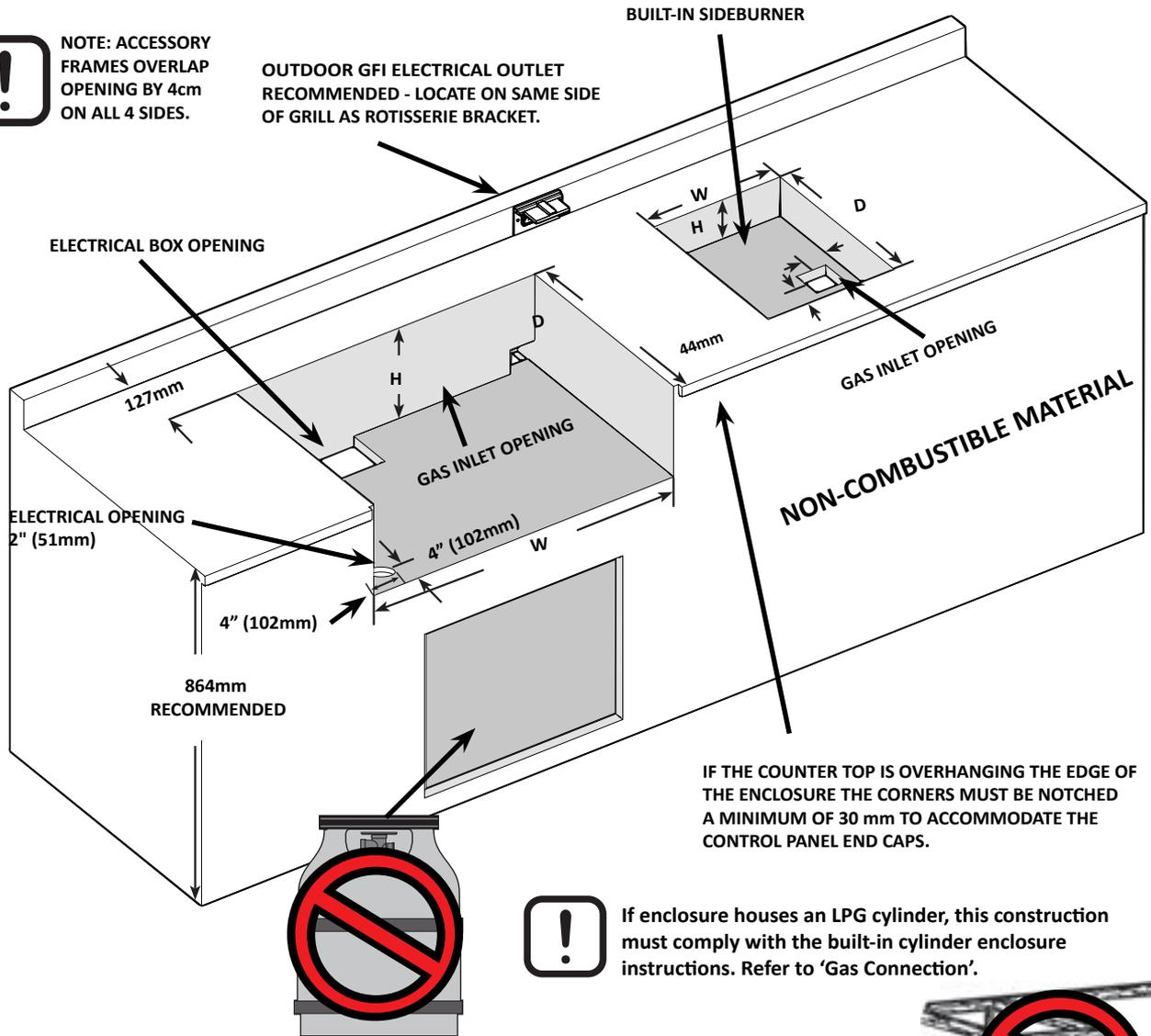
IF THE COUNTER TOP IS OVERHANGING THE EDGE OF THE ENCLOSURE THE CORNERS MUST BE NOTCHED A MINIMUM OF 30 mm TO ACCOMMODATE THE CONTROL PANEL END CAPS.
